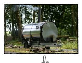
The retort is then lit and fed with scrap wood until it reaches 375 C. At this point the gases are hot enough to be lit and are then redirected into the fire box (outer chamber of the retort) where they are reburnt, further heating the charcoal in the inner chamber.
